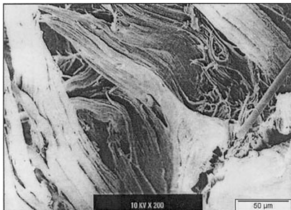
Figure 9 Scanning electron micrographs of tensile fracture surfaces of DCP-treated SGRP (50/50, sisal-glass) composite.
