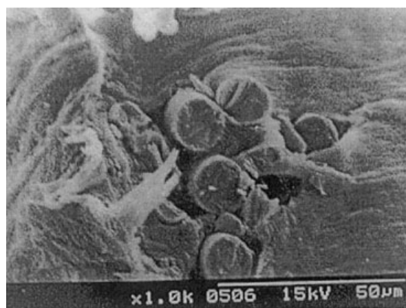
Figure 8 Scanning electron micrographs of tensile fracture surfaces of silane-treated SGRP (50/50, sisal-glass) composite.
